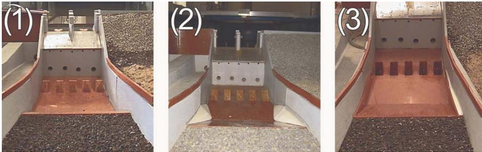
Figure 9. Upstream view of the basin bottom with five baffle blocks laid in one row and variants of modifications of basin walls: (1) original proposal, (2) conical elements, (3) anchored walls
