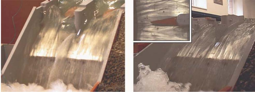
Figure 7. Deformation of the level arising behind the end of the middle pier and its elimination by the NACA profile when  $Q = 610 \text{ m}^3 \cdot \text{s}^{-1}$
