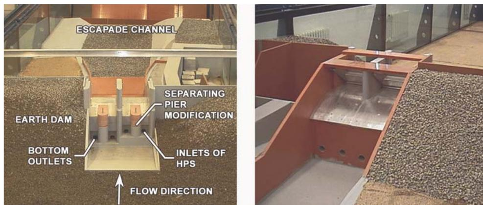
**Figure 2.** Downstream and upstream view of a model of the Znojmo dam spillway block
